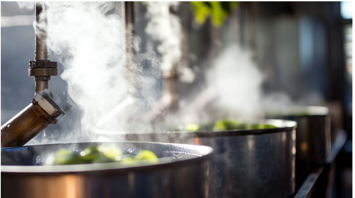
Steam distillation process employed in making Manuka essential oil
